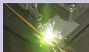
Comparison of the process stability and tendency for droplet emission for steel and aluminum during welding with high brilliance solid-state lasers, left: without (left) and with high frequency beam oscillation (right), ( V_s = 1 \text{ ml/min} , P_L = 1800 \text{ W} , circle = 200 \mu\text{m} , f = 4 \text{ kHz} )
