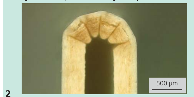
Folding result with optimized scratch geometry
