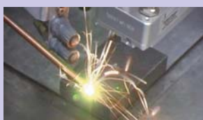
Comparison of the process stability and tendency for droplet emission for steel and aluminum during welding with high brilliance solid-state lasers, left: without (left) and with high frequency beam oscillation (right), ( V_s = 1 \text{ ml/min} , P_L = 1800 \text{ W} , circle = 200 \mu\text{m} , f = 4 \text{ kHz} )
